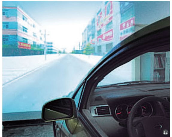
汽车驾驶辅助系统硬件在环仿真试验台 ⑪-⑬ Hardware-in-the-Loop Simulator for Driver Assistant System
